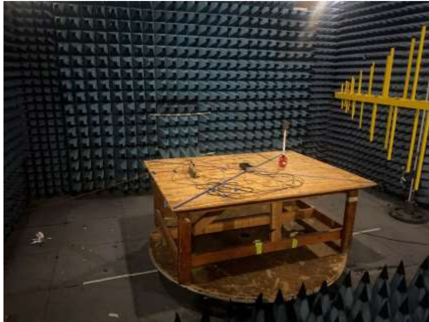
Figure 18. Radiated Immunity, (80 MHz – 1 GHz) Test Setup
