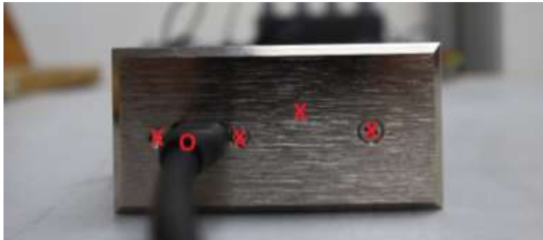
Figure 12. Electrostatic Discharge, Rear of EUT
