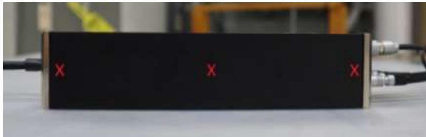
Figure 13. Electrostatic Discharge, Left of EUT
