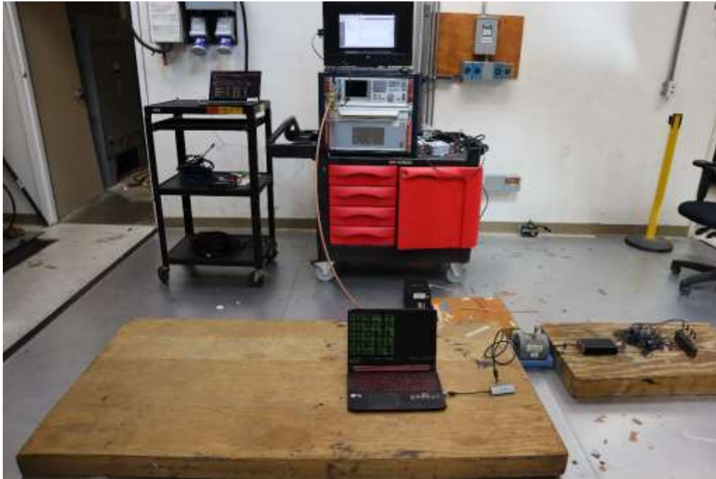
Figure 21. Conducted Immunity, (USB-C) Test Setup
