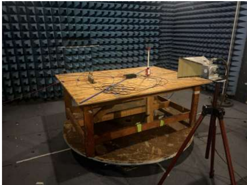
Figure 19. Radiated Immunity, (Above 1 GHz) Test Setup
