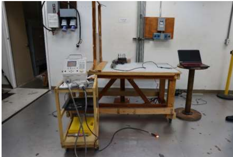
Figure 17. Electrostatic Discharge, Test Setup
