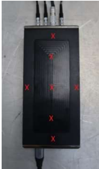
Figure 15. Electrostatic Discharge, Top of EUT
