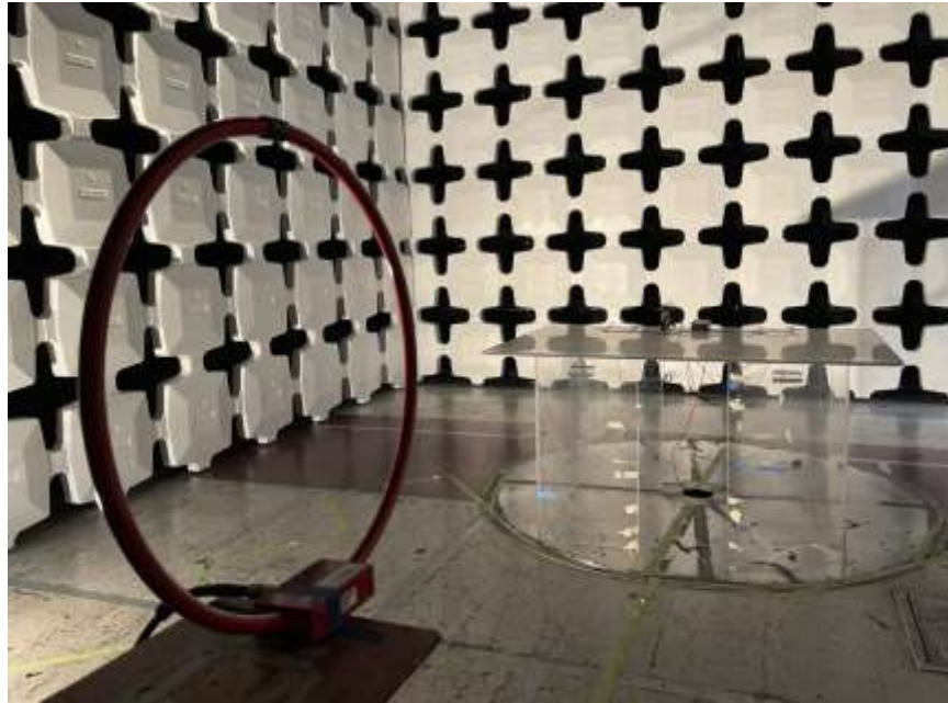
Figure 9. Radiated Emissions, (125 kHz – 30MHz, Y) Test Setup
