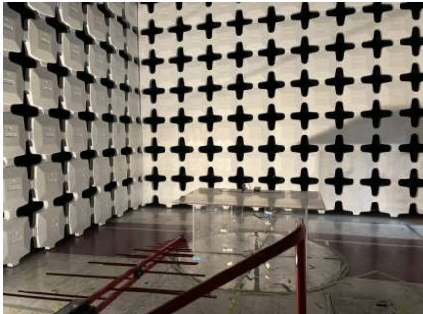
Figure 10. Radiated Emissions, (30 MHz – 1GHz, Horizontal) Test Setup
