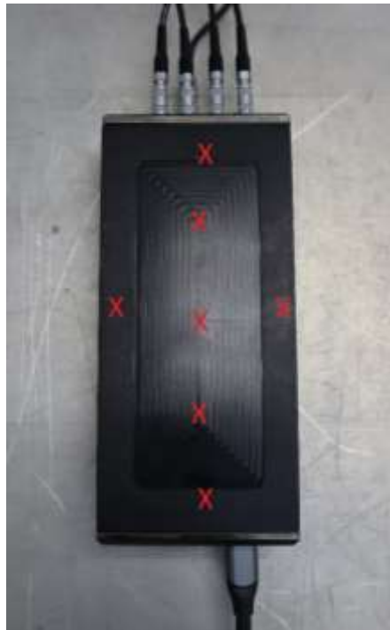
Figure 16. Electrostatic Discharge, Bottom of EUT
